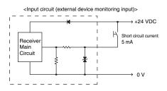
\* The light emission stops when opening the test input line or applying voltage of 0 V to 1/2 Vs to the test input line.
