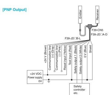
Controllers connectable with PNP output F3SJ series
