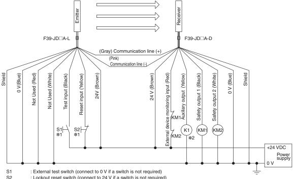
: Lockout reset switch (connect to 24 V if a switch is not required) KM1, KM2: Safety relay with force-guided contact (G7SA) or magnetic contactor
