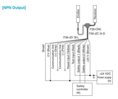
Controller connectable with NPN output F3SJ series
