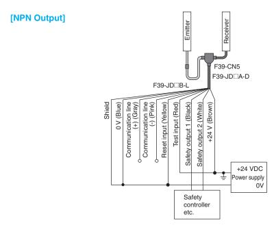
Controller connectable with NPN output F3SJ series
