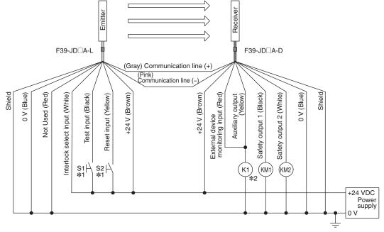
S1 : External test switch (connect to 0 V if a switch is not required)
