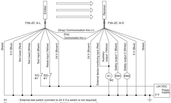
S2 : Lockout reset switch (connect to 24 V if a switch is not required)
