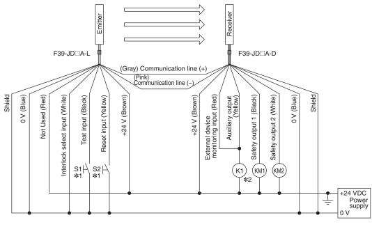
: External test switch (connect to 24 V if a switch is not required)
