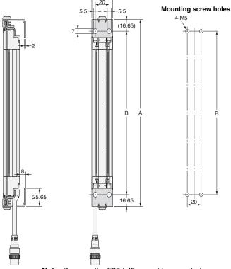
Note: Because the F39-LJ8 cannot be mounted together with an intermediate bracket, keep the protective height at 600 mm max.
