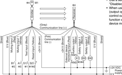
S1 : External test switch (connect to 24 V if a switch is not required) S2
