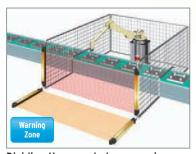
Dividing the zone between seriesconnected sensors
