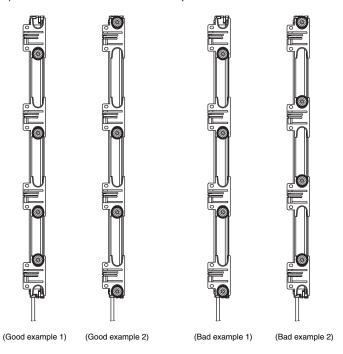
Mount Quick Mount M6 Brackets (or Quick Mount M8 Brackets) according to the mounting positions of the emitter and receiver. The positions of Intermediate Brackets mounted to the emitter and receiver must be aligned with each other.
