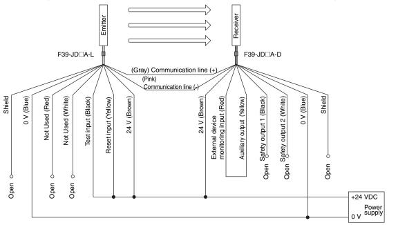
Minimum wiring required to check the operation of the F3SJ-B (Wiring for deactivated external device monitoring) (F3SJ-B COTS) [PNP Output]
